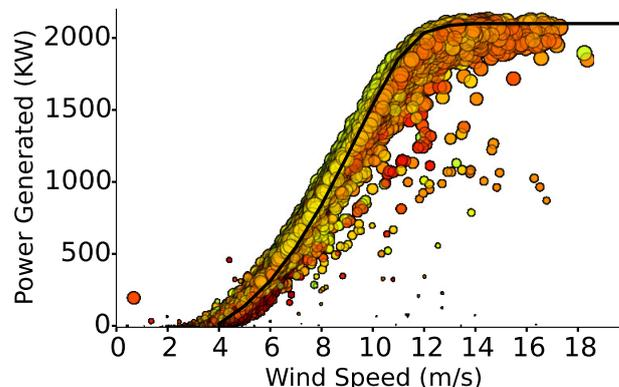
Figure 1: Power generated vs wind speed; Area of the circle represents average time per 10 minutes for which each turbine was operational; color indicates environmental temperature with darker shade representing higher temperature.
